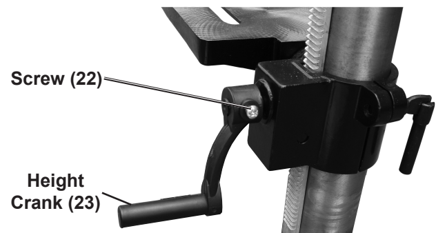
Figure D: Installing Height Crank
