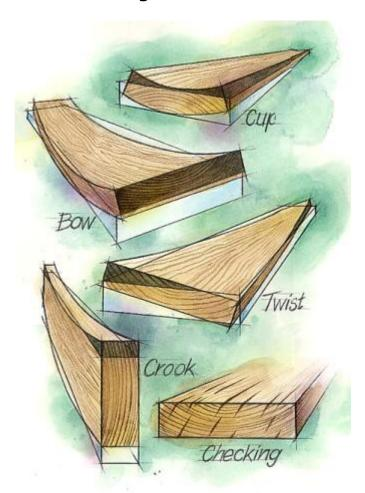
**What shrinkage does to wood** Woodworkers call the change in shape of a piece of wood **warp**. And it takes several common forms, all of which distort the wood. A board has **cup** when it is no longer flat from edge to edge. Cup always occurs in the opposite direction of a flatsawn board's annual growth rings.
