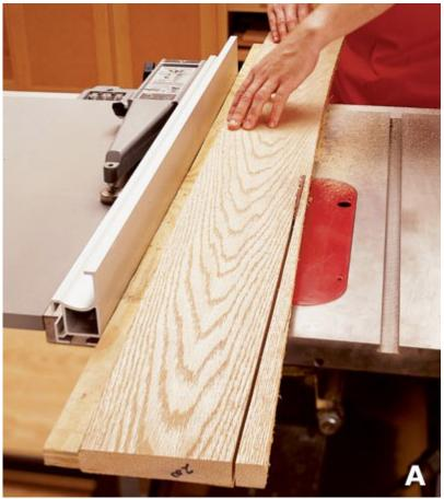
To put a straight edge on a crooked board, stick it on a long, straight carrier,
