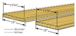
Quartersawn lumber is more stable than plain-sawn, expanding only half as much across its width. Additionally, quartersawn boards remain relatively flat, while plain-sawn boards tend to cup when they expand and contract.\*
