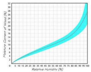
The moisture content of the wood varies with the relative humidity of the surrounding air, as this chart shows. Once the wood has been dried, the moisture content never again rises above 28 percent (its fiber saturation point) from the effects of humidity alone. For this to happen, the wood must be immersed in water.\*
