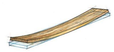
Bow: A board that rocks from end to end when laid on one face.
