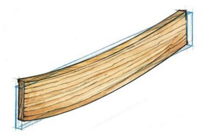
Crook: A board that rocks from end to end when laid on one edge.
