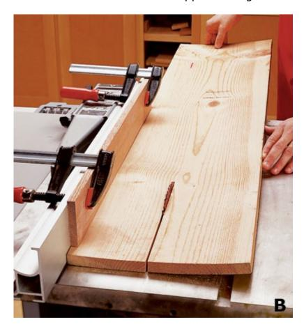
Rip cupped boards with the convex face against the saw table. A scrap clamped to the fence guides the workpiece and holds the portion being cut flatly against the table.
