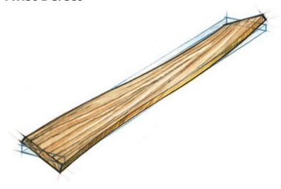
Twist: A board that rests on opposite diagonal corners when laid on one face.
