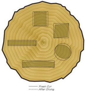
Because of the difference in tangential and radial movement, boards change shape as they expand and contract. The way in which they change depends on how they are cut from the tree.\*
