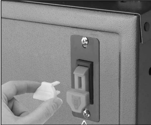
Figure 12. Removing lock-out key from switch.
