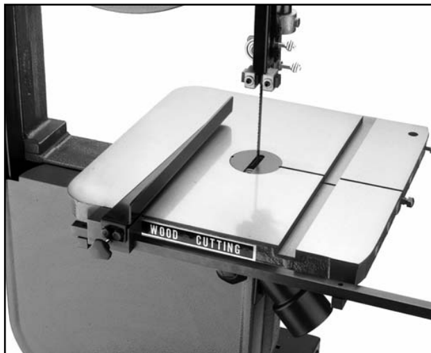
Figure 22. Fence in position.
