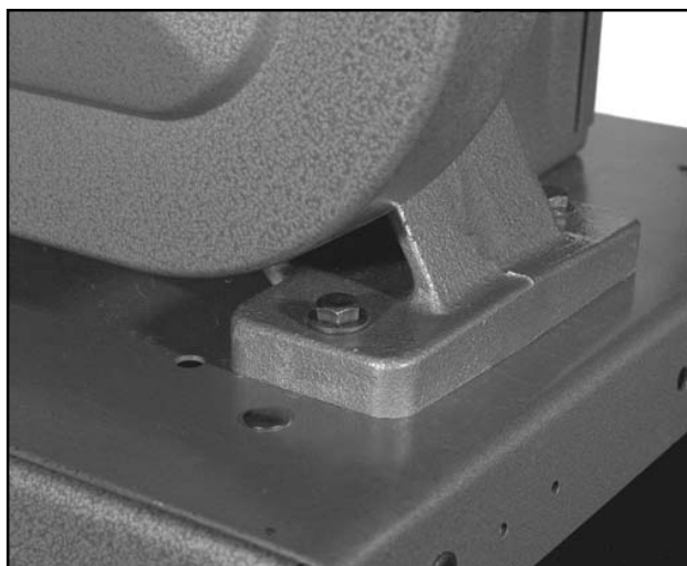
Figure 14. Loosely fasten to base.
