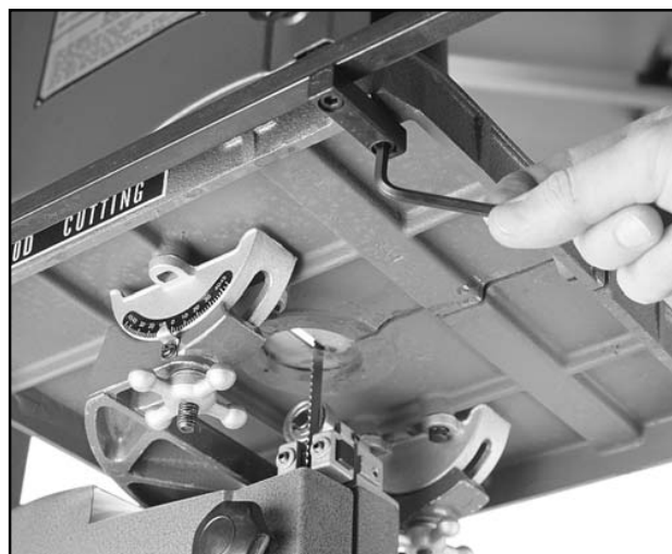
Figure 21. Fence rail bracket attachment.
