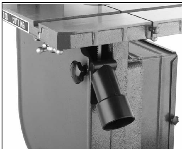
Figure 20. Dust port in place.
