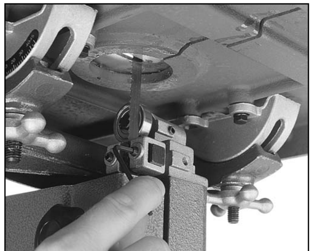
Figure 26. Lower blade guide assembly.
