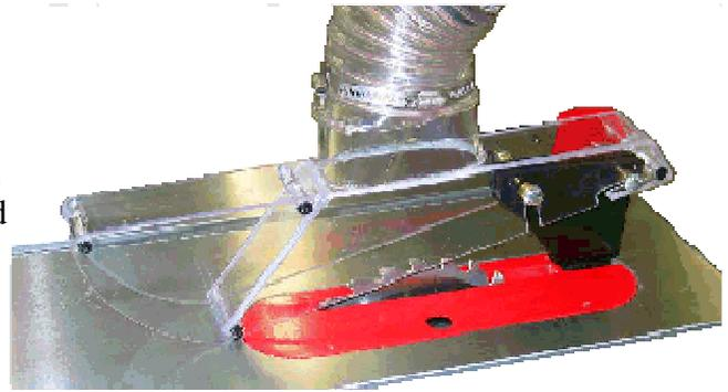
originally thought I could get by with using my existing 2.5" port on my splitter mounted blade guard on my table saw. The CFM Requirements chart showed I needed at least 350 CFM, but testing the airflow with that smaller port showed only 183 CFM. In short, for good fine dust collection we almost always have to rebuild our hoods and use larger ports.
