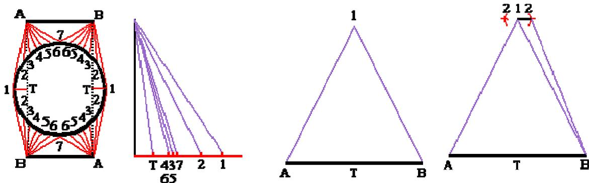
9. The diagonal for each of these right triangles is the actual length of the line used to layout the metal cutting/folding diagram. You can either use math to calculate the lengths of these fold lines or you can get them by drawing a right angle. This angle forms a right triangle as tall as the height of the fitting and base
