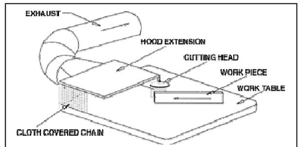
To overcome this problem, a hood extension with a flexible face opening is added. The flexible face opening consists of cloth-covered chains that allow the wood to pass through, but stops the wood dust particles. The extension also increases the hood face velocity by minimizing the open face area.
