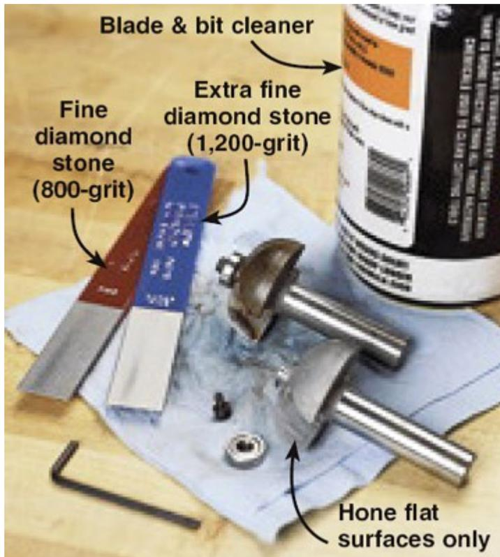
A dull bit cuts poorly and builds up heat doing so. If you can run the cutter over your fingernail without shearing off a shaving, then your bit needs sharpening.
