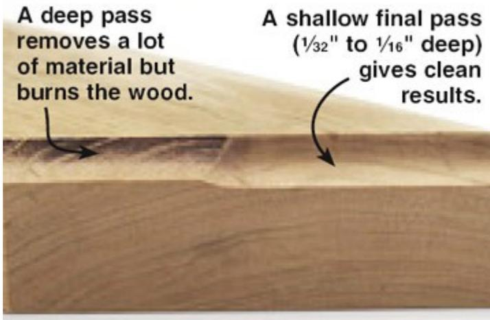
Powerful routers and sharp carbide-tipped bits are capable of hogging out large cuts in even the hardest of woods. But doing so stresses the bit, causes tear-out, and leads to burning. When removing more than 1/4" of material, make multiple shallow passes....
