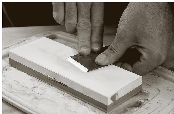
*IF YOU DON'T POLISH THE backside of your newly acquired chisels and plane irons, your cutting edges will always be jagged and easily dulled. You need to polish just the area up by the cutting edge. This is a process you'll only have to do once.*
