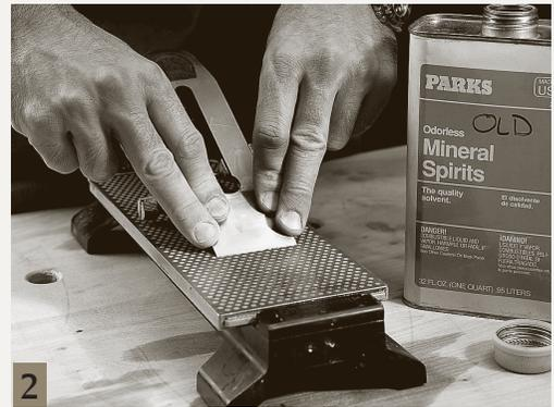
2 FLAT-GRINDING YOUR CUTTING BEVEL SHOULD *not* take long on a coarse diamond stone. If you’re having trouble gauging your progress, color the cutting bevel with a permanent marker and you’ll get a quick snapshot of where you stand.
