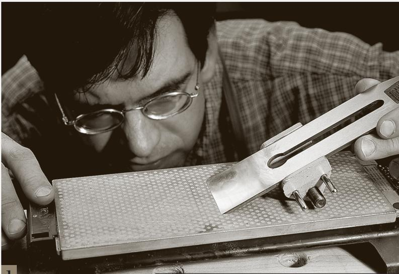
1 TO BEGIN GRINDING YOUR EDGE, put the tool in your honing guide and adjust it until the cutting bevel is flat on your stone. Eyeball it at first. After a couple passes on the stone you’ll know if you’re off or not.
